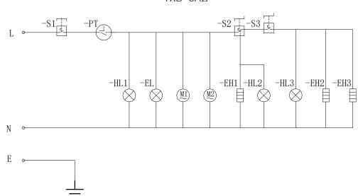
EH1---Upper Heater EH2、EH3--- Main Heater EL---Inside Lamp M1、M2---Convection fan S3---Thermostat for Main Heater S2---Thermostat for Upper Heater S1-Hi-limit PT---Timer HL1~HL4---Pilot Light
