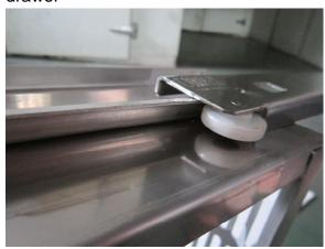
C. Lift drawer and remove from channel.
