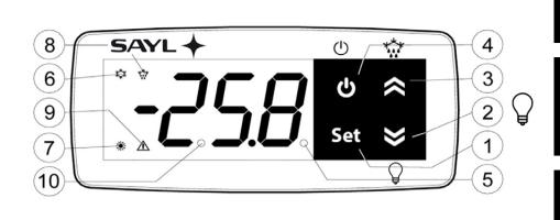
**Key 1 -** SET: Sets the set point (Temp work) and operating parameters.
