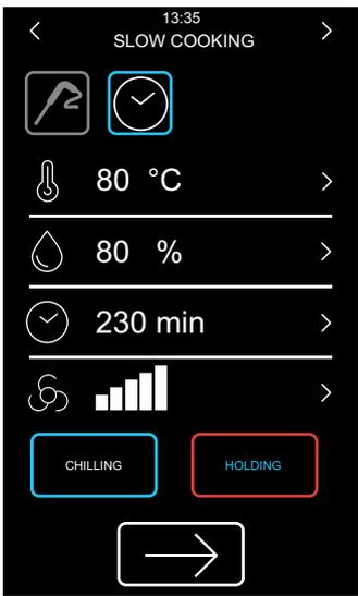
Two specific areas located in the lower part of the screen allow adding an extra phase:
