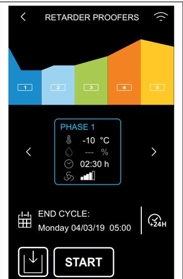
In case set end time is later than the sum of each phase time, the controller will automatically increase storage time (phase 2) to fill in the time gap.
