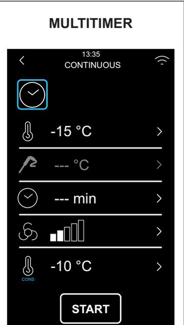
Cycle is started by pushing the
