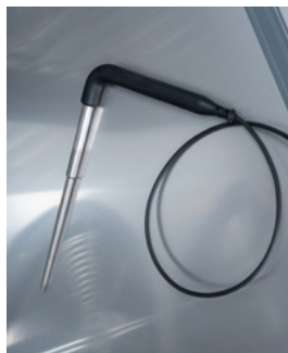
Angled probe easier to hold.
