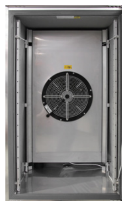
Double air flow evaporator back
