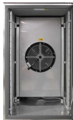
Double air flow evaporator back
