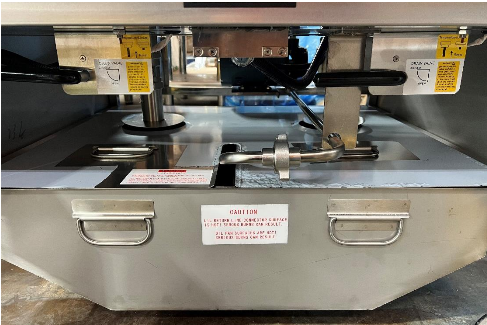
Figure 8: Oil Collection Tank
