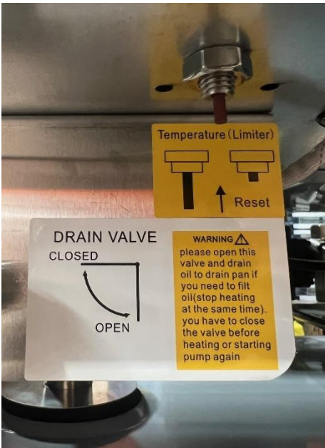
Figure 14: Temperature Reset Button
