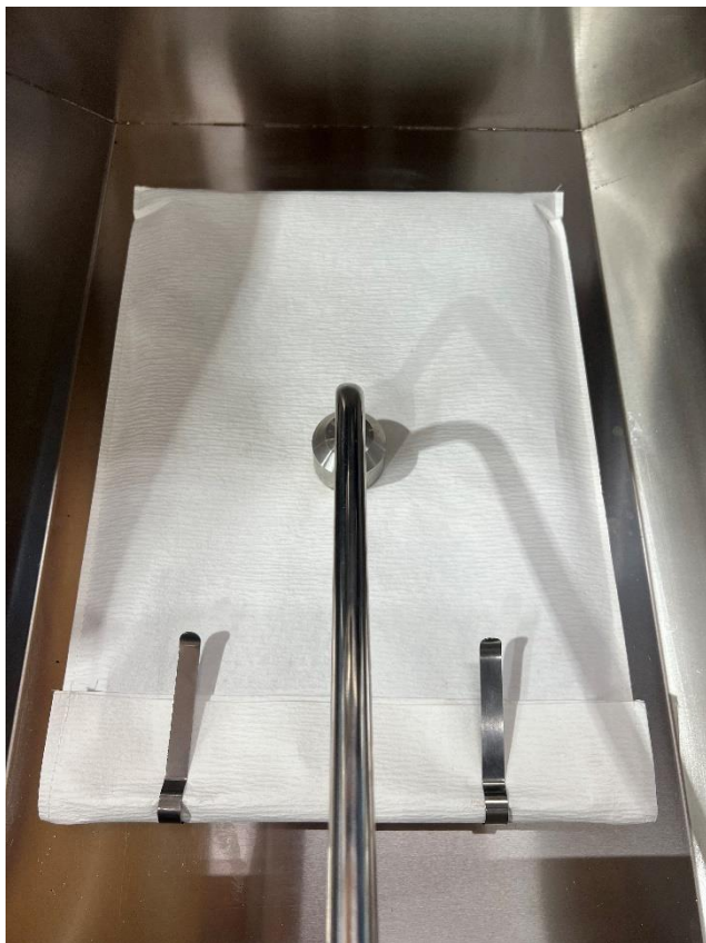
Figure 12: Filter Envelope, Standpipe and Filter Clips
