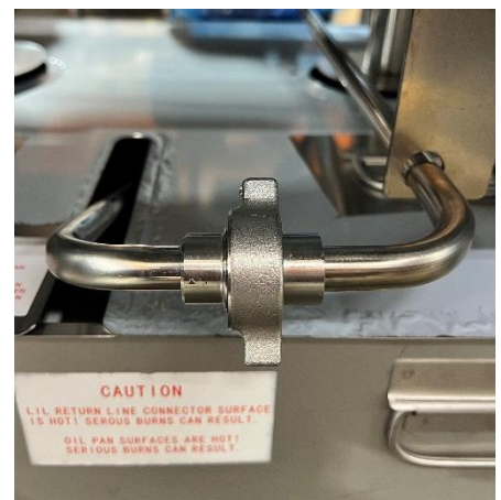
Figure 10: Filter Union Connection
