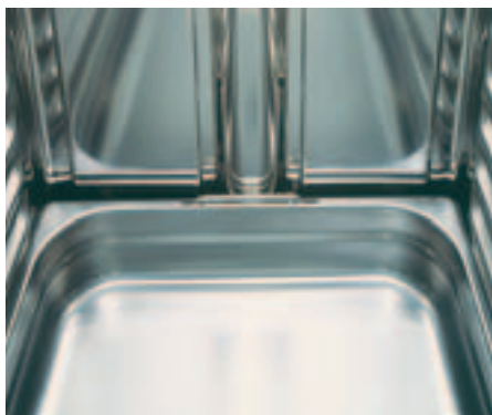
Easy to heat: Air circulation heating with even heat distribution thanks to chimney effect (the ends of the inserted Gastronorm containers stop before the back wall and create a chimney).
