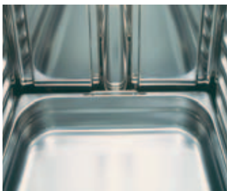
Easy to heat: Air circulation heating with even heat distribution thanks to chimney effect (the ends of the inserted Gastronorm containers stop before the back wall and create a chimney).
