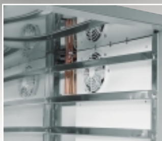
Evaporator in centre in 2-part version
