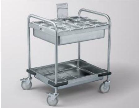
Spice trolley 2 deep-drawn welded trays. 12 spice holders with self-closing, transparent plastic lids. Below, 8 divisions 120 x 120 mm. 4 corner bumpers. Rustproof castors in accordance with DIN 18867, Part 8.
