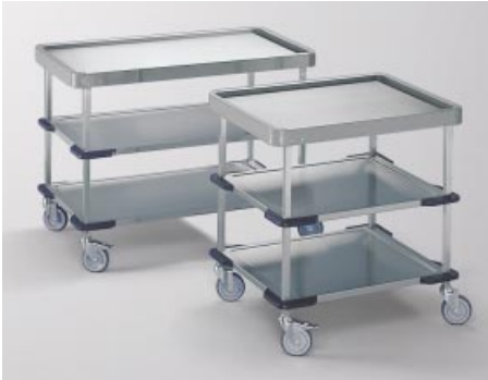
Sub-frame in square tube material. 2 deep-drawn shelves with raised edges, welded-in with 4 corner bumpers each.
