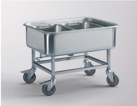
Potato and vegetable washing trolley Stainless steel bowl, deep-drawn with beaded edge, lever drain outlet with basket strainer 2". Suitable for: 2 x GN containers 11194 K. Wells: 750 x 560 x 230 mm. Rustproof castors in accordance with DIN 18867, Part 8.
