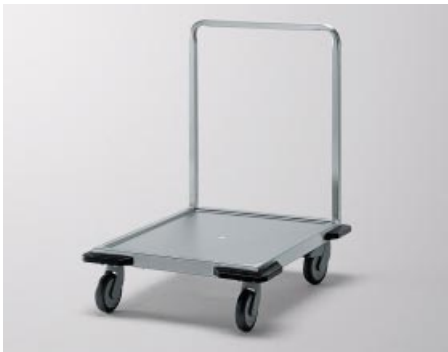
Platform trolley for baskets with pushing handle in stainless steel. 4 corner bumpers. Platform with stopping edge and drainage bore-hole. Rustproof castors in accor- dance with DIN 18867, Part 8. 2 swivel castors, 2 swivel castors with brake ø 125 mm.
