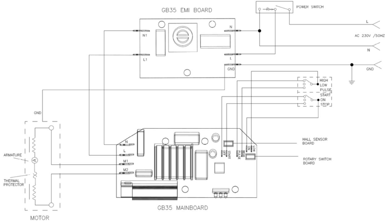
GB35 SCHEMATIC WIRING DIAGRAM
