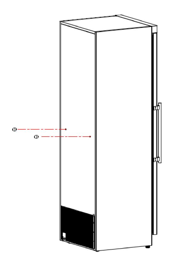
The rubber spacer must be screwed into the back side of the cabinets as showed above to ensure proper distance especially when the unit is placed against the wall. Failure to do so may void warranty and cause failures to the compressor.
