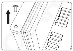
3. Remove the right upper hinge and install it on the left side. Afterwards, install the hinge sleeve onto the hinge.
