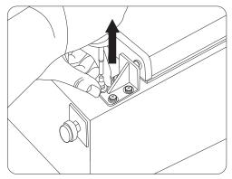
2. Remove the door from the right upper hinge. Then remove the hinge sleeve from the door top.
